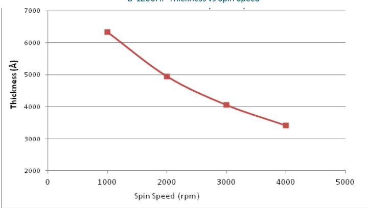
B-1200HP Thickness vs Spin Speed
