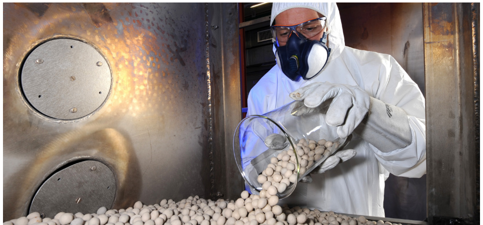
Testing ceramic materials for use as thermal storage media
